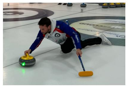
The delivery can be videotaped and the position of the laser on the rock will indicate any movements off the line of delivery.
