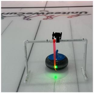
The curling target is positioned beyond the near hog line before the break point. The laser should shine on the ribbon (a rock can be placed in the middle of the target to confirm it is positioned correctly. Curlers can videotape themselves delivering with a smart phone placed on the phone mount of the target.
