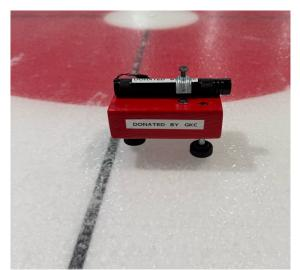
A laser is used to provide a target at the far end of the sheet of ice. It is positioned to shine on the middle of the rock in front of the hack.
